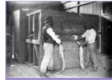
On its return from the drying fields the fibre was “scutched”. Each man held a hank of fibre which was beaten by a revolving paddle wheel. About half of the hank would be blown out of the back as “tow”, the remaining long fibre baled for export or used for local rope production.
